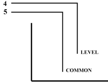
**2 Electrodes - Conductive Tank**
